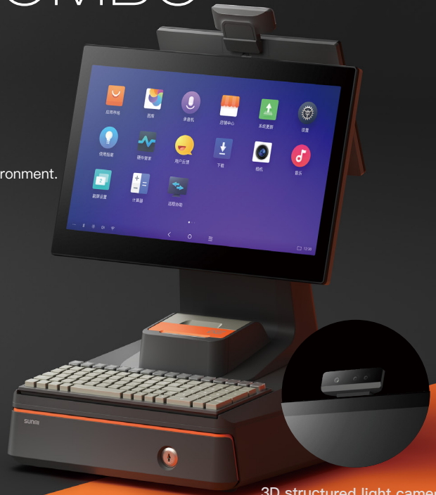
3D structured light camera supports facial recognition payment
